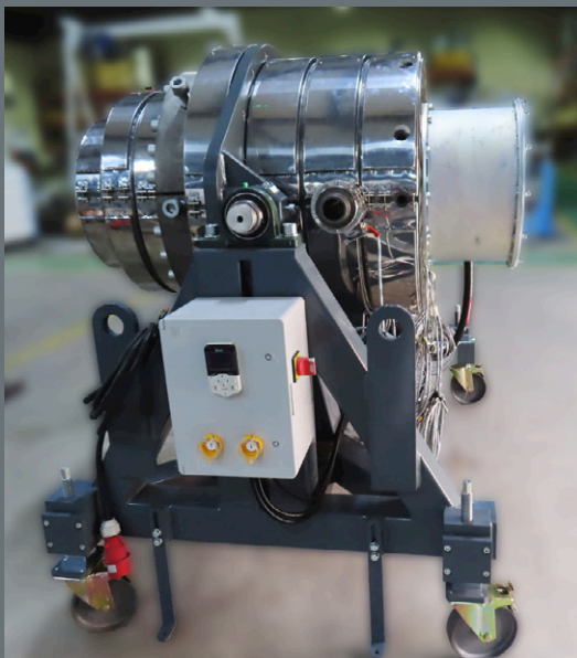
PO 4 400 CR – 4 layer cross head for barrier pipes
