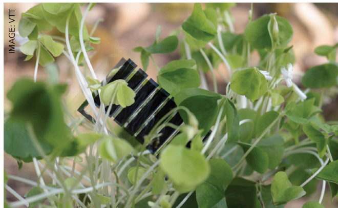
Above: VTT's degradable solar cell can be used to monitor agricultural crops
