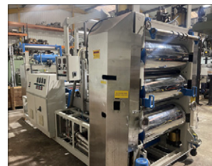
1040mm wide Welex 3 roll polishing stack
