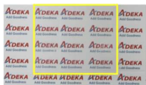
Test piece (1 mm) made of Polypropylene with 0.1% ADK TRANSPAREX™
