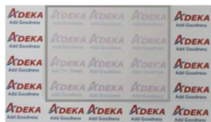
Polypropylene test piece (1 mm) without the addition of a clarifier
