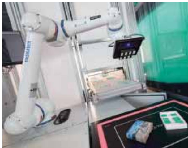
After a linear Multilift V 30 robot places 32 dominoes on a conveyor belt, a cobot takes over the subsequent packaging of the complete ready-to-use set. Arburg GmbH + Co KG photo
