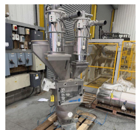
4 component Colortronic gravimetric blender
