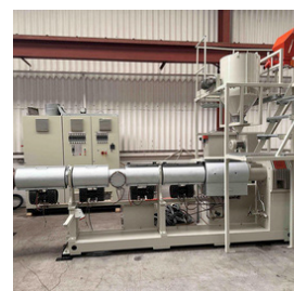
120mm Battenfeld Single Screw Extruder
