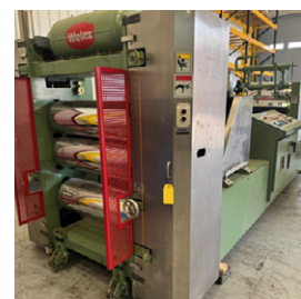
890mm x 300mm Welex 3 roll polishing stack
