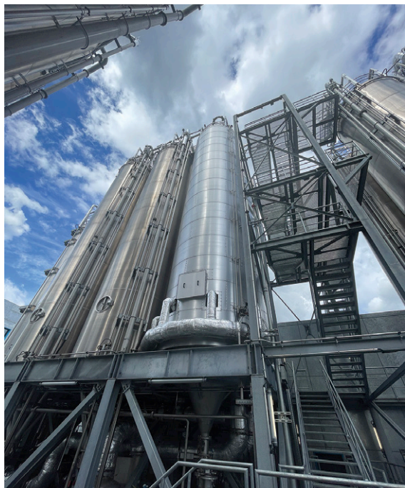
Coperion's EcoFresh silo degassing system (pictured) and its twin screw extruders have received a Letter of No Objection from the FDA and are therefore suitable for the production of food-grade HDPE and PP recyclates
